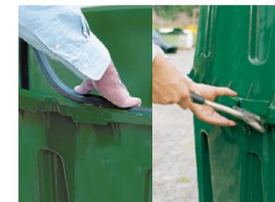
**Insert the seal. Connect the tank halves.**
